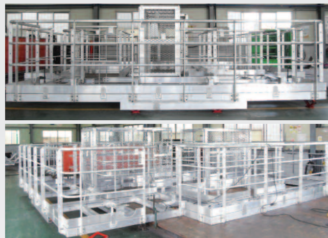
Platform(aluminum) and Vertical ladder(aluminum) installed on derrick for drilling.
