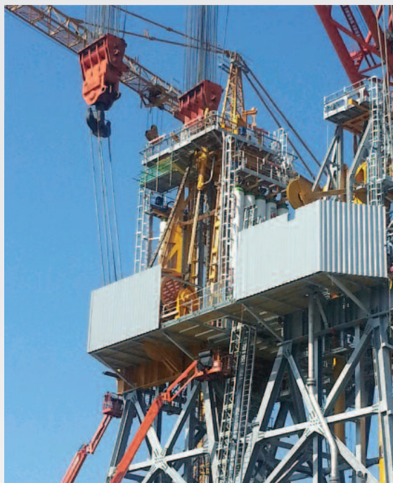
Platform(aluminum) and Vertical ladder(aluminum) installed on derrick for drilling.
